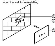
6. Install the shower to the right connecting pipes, tighten clockwisethe M4 screw with S2.5 Allen key
