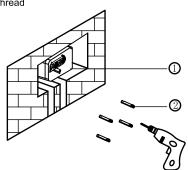
3、 Make sure that the wall mounted body box 15mm protruding out the tile on the wall. Please remove the extra 15mm when the showerinstalled, make sure it is flat with the wall
